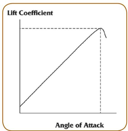
Figure 4: Lift coefficient versus AOA showing stall
