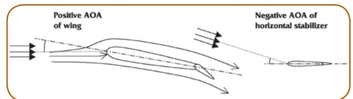
Figure 3: AOA at wing and horizontal stabilizer
