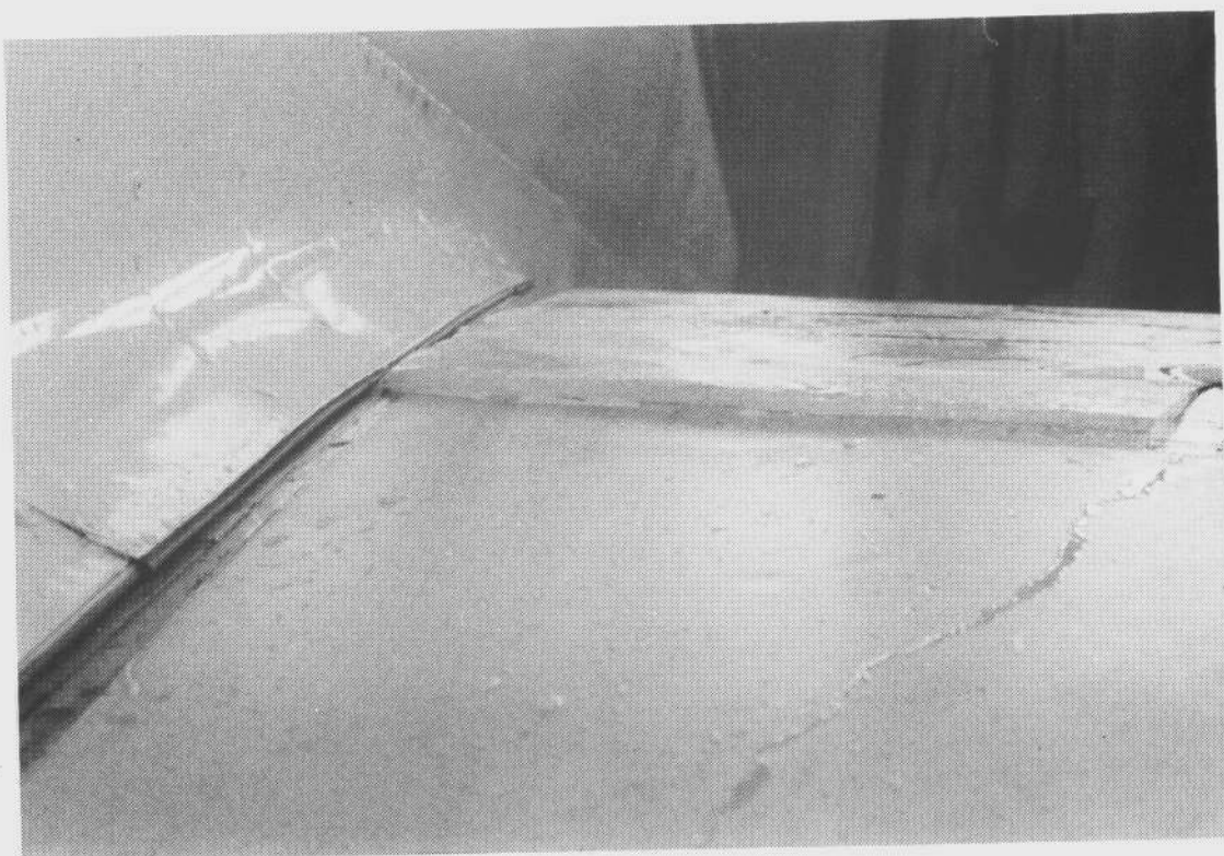
1. Ice layer on the right wing, seen from the back of the wing. Observe the dent at the rear wing spar. (Photographed in the hangar).
