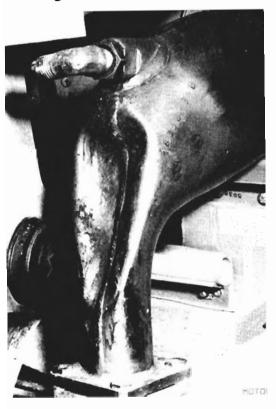
Fissure in welded seam
