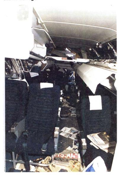
open them immediately after the crash. The rear service door could be opened later. Three of the four emergency exit windows were open. According to information from witnesses, the rear right exit was blocked with loose seats, cabin luggage etc.
