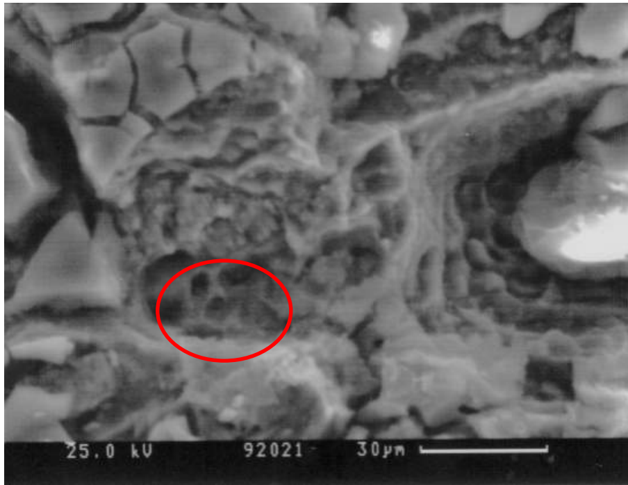
Figure 1.16-5 SEM examination showing the dimple structure (790X) ◦
