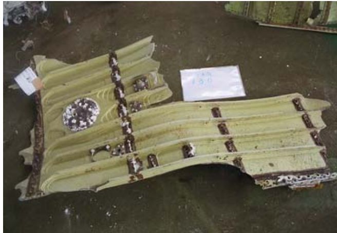
Figure 1.12-6 Wing root skin (bottom of fuel tank)
