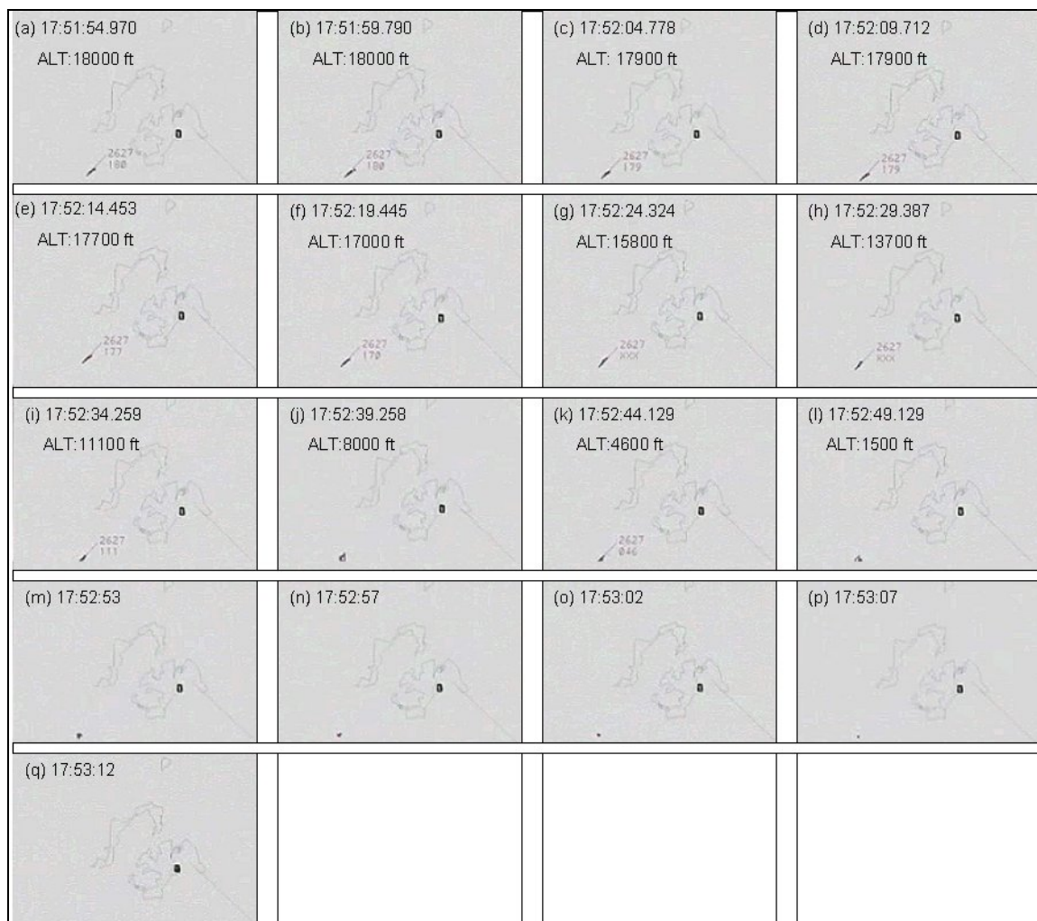
Figure 1.18-5 Secondary and primary radar returns recorded by the ATAS ( from TACC )
