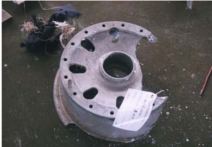
Figure 1.12-20 Broken wheel hub
