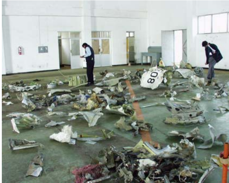
Figure 1.18-11 Underwater wreckage recovered by trawling operation
