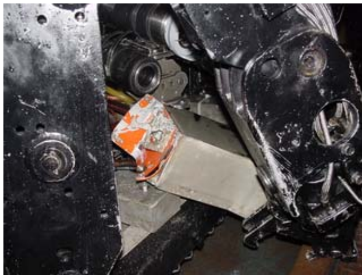
Figure 1.18-27 CVR recovered by ROV
