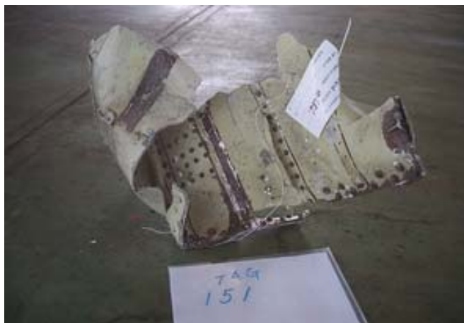
Figure 1.12-8 Wing trailing edge structure
