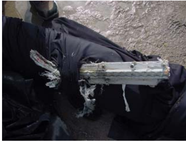
Figure 1.12-31 One roll of cloth was protruded by floor structure
