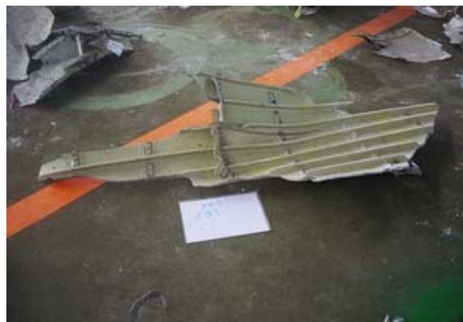
Figure 1.12-7 Wing tip structure (top of fuel tank)
