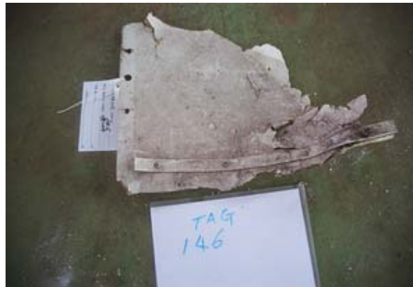
Figure 1.12-5 Cargo compartment partition
