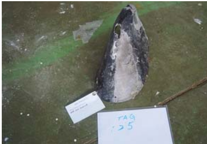
Figure 1.12-23 Power plant tail cone
