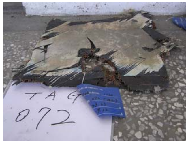
Figure 1.12-10 Flap honeycomb structure
