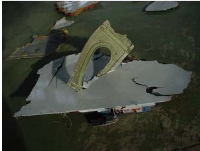
Figure 1.12-15 Window frame stuck into rudder
