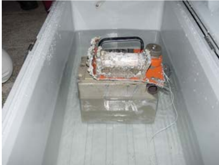
Figure 1.18-26 FDR close view while recovered
