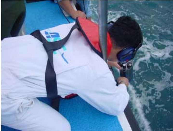
Figure 1.18-17 Search flight recorders with pinger receiver
