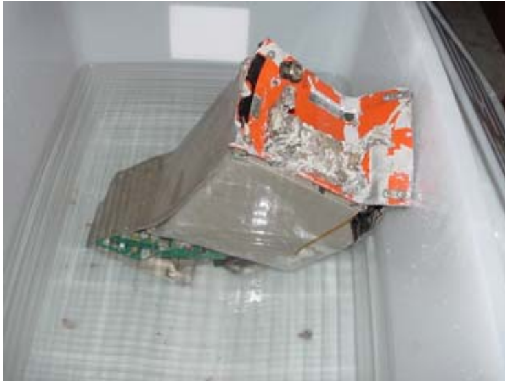
Figure 1.18-28 CVR closed view while recovered
