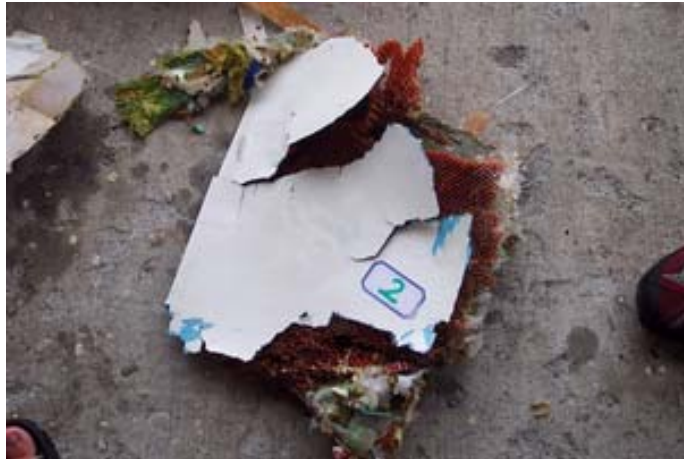
Figure 1.12-12 Vertical stabilizer honeycomb structure
