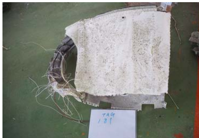
Figure 1.12-11 Flap leading edge structure
