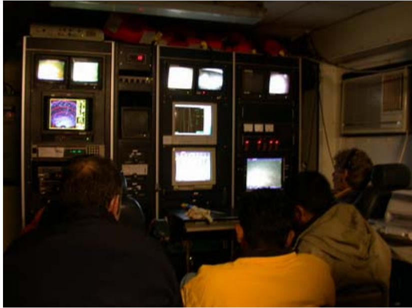
Figure 1.18-24 Visual check with ROV video camera and forward sonar scanning
